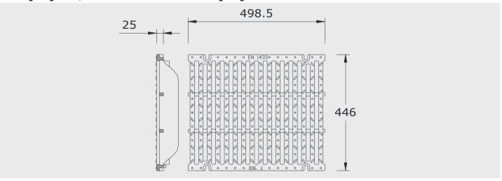
Class F900 to EN 1433, ductile iron with 4-fold-bolted channel grating securement
